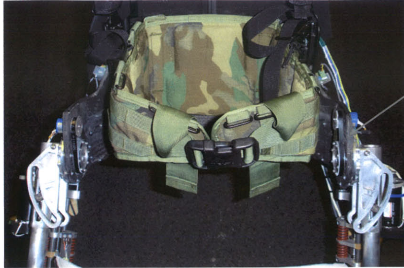
Figure 4.5 Hip angle sensing was done by means of a timing belt and pulley with a 2:1 reduction on a Bourne rotary pot. The belt system was attached to the hip joint on the inside of the harness as shown.
